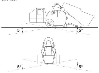
The machine must be placed at that point on the jobsite where you can take best advantage of the hoses' operating range.
