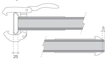
Hoses Ø 65 x 84 - length of 10 or 20 meters for max. pumpable granulometry of 0 - 15 mm.
