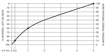
Use, for instance, sand with granulometry: 1/3 from 0 to 1 mm; 1/3 from 1 to 4 mm; 1/3 from 4 to 8 mm.
