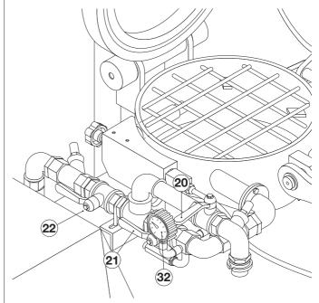
Open to 3/4 the cock **(22)** which regulates the air flow to the material outlet collector and open 1/4 of the way the cock **(21)** which regulates the air flow to the material vessel.
