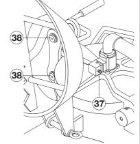
• <u>Loading bucket</u> (EB version) Grease the 4 loading bucket greasing points.
