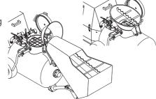
• Load 50% of the sand, than 100% of the binder (cement), then all the water and finally the remaining 50% of sand. For the version with loading bucket (EB version), the material is loaded into the loading bucket; then trough the lever for the loading bucket control, start to unload the material into the vessel.
