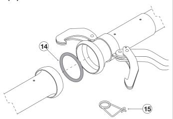
lock the levers tightly with the safety stop (15).
