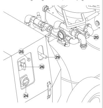
If the lamp goes out during the starting, it means that the voltage is not sufficient.
