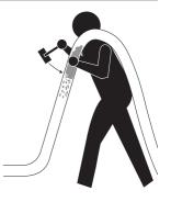
Never disconnect hoses or delivery hopper, unless you are not completely sure that there is no pressure (0 bar) in hoses and vessel.
