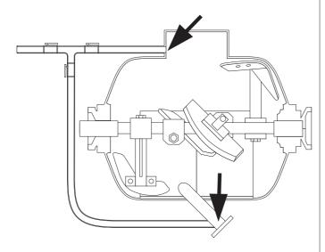
• Insert a suitable washing sponge into the front end of the material delivery hose and connect the hose to the machine.
