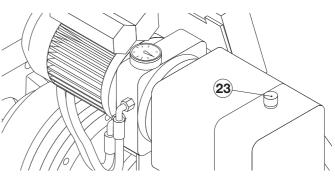
Check oil level and eventually fill up with lowered loading bucket .
