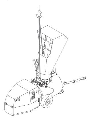
The loading bucket must be in vertical position and locked with the red painted safety bar.
