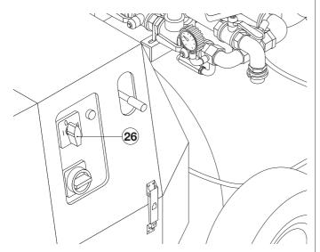
The material vessel pressure lows quickly to zero. Open the hatchway.
