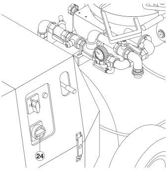
Disconnect the air delivery hose from the material delivery collector and check to see that it is clean.
