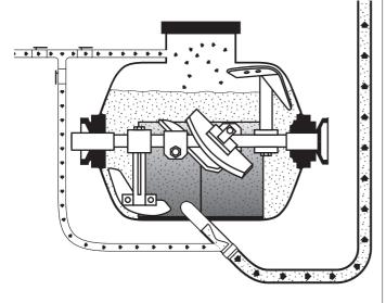
The vessel itself is pressurised through a compressor and the material, pushed through the hose by the paddles towards the outlet collector, is conveyed to its point of use.
